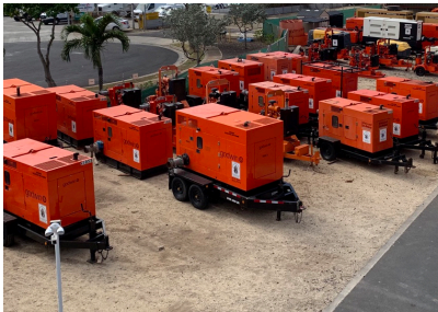
Dri-Prime Pumps for Sewer Bypassing & Dewatering
